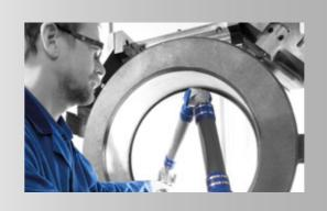
With the three-dimensional measuring system, the valves can be measured and scanned against 3D data and subsequently evaluated and saved on a PC. The measurements are carried out directly in the machine to ensure reliable production processes.
