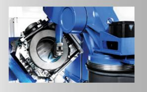
The sealing surface is coated with stellite by a fully automatic welding robot with an integrated measuring system. All CNC programs are developed by our expert in-house programmers. The precise synchronisation of the welding system's eight axes ensures high product quality.
